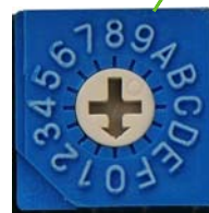
Figure 6) - Rotary switch= CAN address selector (For details see the section 3.2.3 “CAN Address Designation”)
